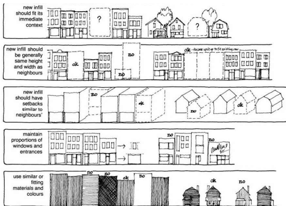
Figure 16: Diagram showing good and bad examples of infill (OHTK, Ministry of Tourism, Culture and Sport of Ontario)
